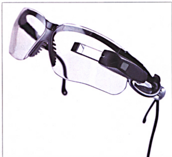
Figure 5. This heads-up display from FLIR systems enhances worker safety by enabling the thermographer to see the infrared image without having to look into an eyepiece or a LCD screen. The technology projects the infrared image onto a pair of safety glasses.
