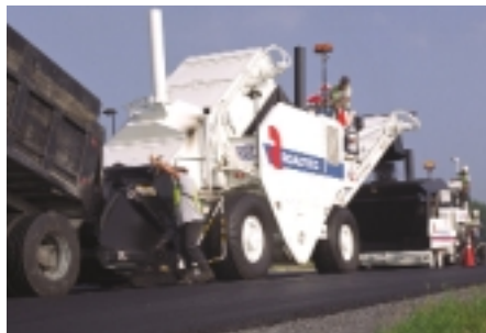
The Shuttle Buggy material transfer vehicle, manufactured by Roadtec.
