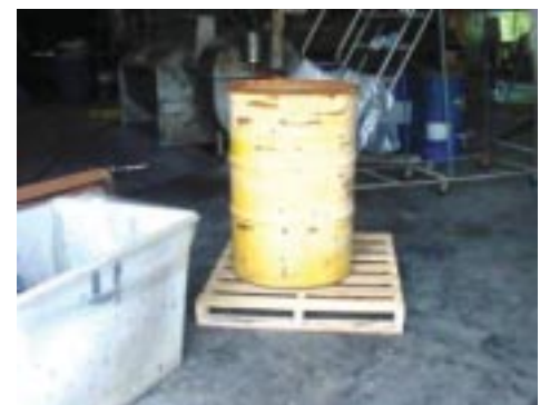
The 55-gallon drum contains the 32-gallon drum of hot sodium hydrosulfite and a quantity of coolant water.
