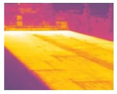
Thermal image indicates a uniform temperature mix, essential for pavement smoothness.
